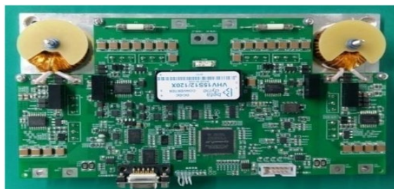
Figure 1 Solar cell power regulator
